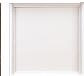
27: Sugar (L) An opaque, clean white finish with a very slight intermittent rub-through along the perimeter edge.
